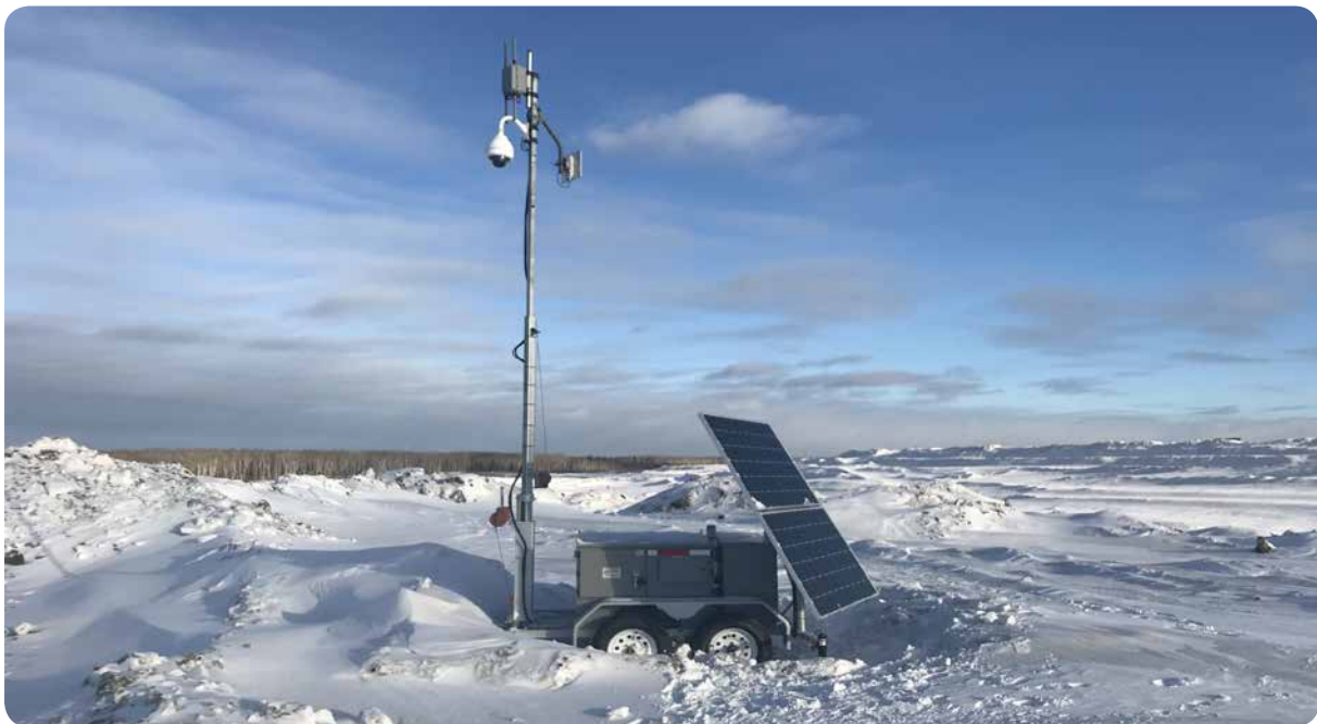
EFOY Pro trailer in use in Canada. Hybrid fuel cell solutions deliver reliable power even in snow and freezing climates.
